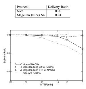
Fig. 5. Lateral-error recovery significantly increases the resilience of multiple-tree protocols (512 end hosts, unlimited bandwidth).
