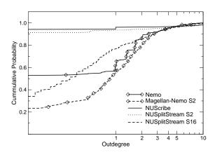
Fig. 8. Physical outdegree is the packet-forwarding capacity, as a fraction of a basic stream rate, contributed by a node. It determines the scalability of an overlay system in bandwidth limited scenarios (512 end hosts, unlimited bandwidth, MTTF=120 min, MTTR=20 min).
