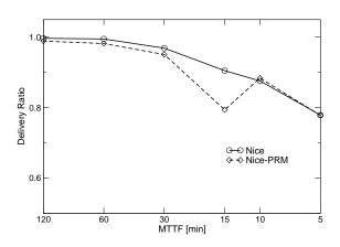
Fig. 2. PRM increases the average delivery ratio for different degrees of churn, specified in terms of MTTF (512 end hosts, unlimited bandwidth). Note that the x-axis crosses at 0.5 delivery ratio.
