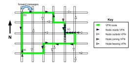
FIGURE 2: Illustration of a simple VFN topology.
