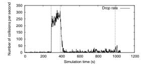
FIGURE 3: Graph depicting the number of packets dropped due to collision when VFN is enabled and temporarily disabled.
