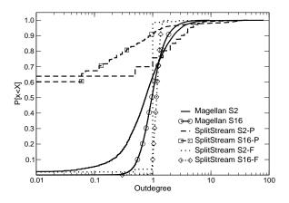
Figure 10. Outdegree CDF (Simulation, high bandwidth scenario). S2-P and S16-P denote performance-optimized tree constructions schemes, i.e. the outdegree is set according to the peer's available bandwidth, while S2-F and S16-F stand for the fair construction scheme, i.e. the outdegree is set equal to the number of stripes.
