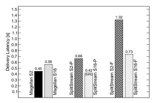
Figure 11. Delivery Latency (Simulation, high bandwidth scenario). S2-P and S16-P denote performance-optimized tree constructions schemes, i.e. the outdegree is set according to the peers available bandwidth, while S2-F and S16-F stand for the fair construction scheme, i.e. the outdegree is set equal to the number of stripes.
