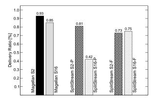
Figure 12. Delivery Ratio with Failures (Simulation, high bandwidth scenario). S2-P and S16-P denote performance-optimized tree constructions schemes, i.e. the outdegree is set according to the peers available bandwidth, while S2-F and S16-F stand for the fair construction scheme, i.e. the outdegree is set equal to the number of stripes.
