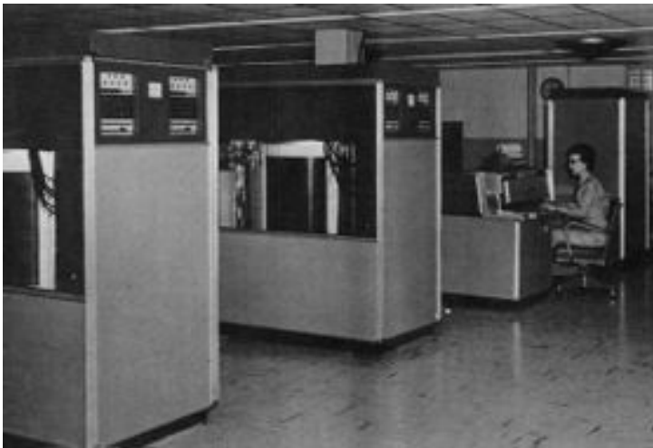
IBM 350 Disk Storage Unit Announced Sep. 4, 1956 5MB
