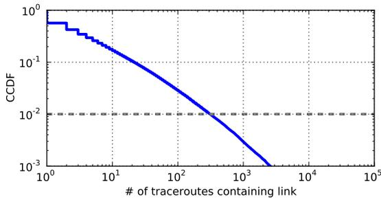
**Figure 6:** CCDF of the number of times each “link” (pair of consecutive IP addresses in a traceroute) appears. We selected the top 1% most popular links as a threshold (dashed gray line) to identify the set of the most popular links.
