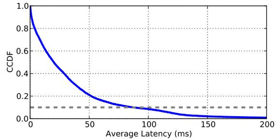
**Figure 7:** CCDF of the latency across the top 1% of popular links (from Fig. 6). To limit our analysis to long-haul links, we selected the top 10% links (greater than 87 ms latency).
