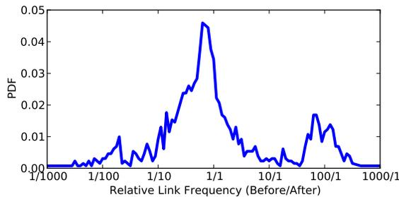
**Figure 10: Probability density function of link popularity ratio between “Before” and “After” traceroute datasets. Most links appear with roughly the same frequency in both periods, corresponding to the peak near 1/1. However, we identify clusters of peaks near 100/1 and 1/100, which correspond to links that significantly decreased or increased in popularity between the two periods.**
