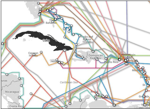
**Figure 1: Map of submarine cables in the Caribbean.** (Source: <http://www.submarinecablemap.com/>)
