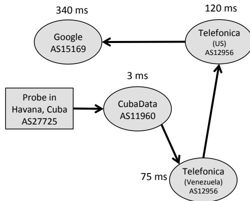
**Figure 4: Traceroute from Atlas probe in Cuba to google.com.** The latencies represent the RTT at each hop. Hops with similar RTT in the same AS have been omitted.
