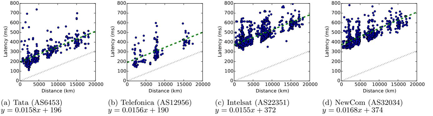
**Figure 5:** RTT from Namehelp users to prefixes in Cuba by distance. Paths are split across figures based on the network immediately prior to CubaData (AS11960). Traffic through Tata’s and Telefonica’s network reach Cuba via the ALBA-1 submarine cable while IntelSat and NewCom use satellite connections. The equation below each figure represents the linear regression between distance and RTT.
