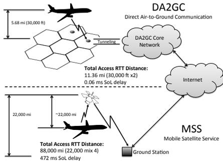
**Figure 1: Technology alternatives for IFC. Direct Air-to-Ground Communication (DA2GC) utilizes cellular connectivity to ground stations, and Mobile Satellite Service (MSS) connects through satellite relays.**
