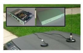
Figure 1. GPS and radio antennas installed on the roof of a vehicle. The car's windshield is visible in the lower left-hand corner of the image. The inset shows the internal hardware and exterior of the Soekris machine.
